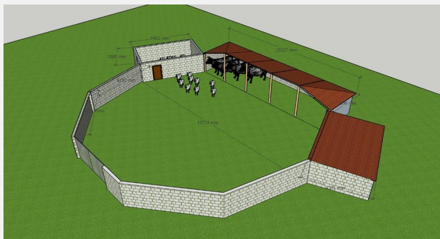
Figure 5: Basic design of winter shelter for animals
