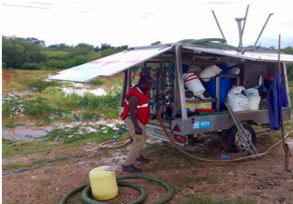
Water purification using the SETA ERU is being used in a camp set-up.
